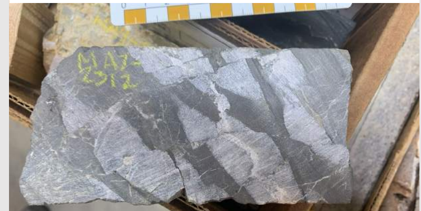
Drill Hole MA22C-007 intersected 23 ft. @ 0.210 oz/ton Au incl. 4.7 ft. @ 0.357 oz/ton Au
